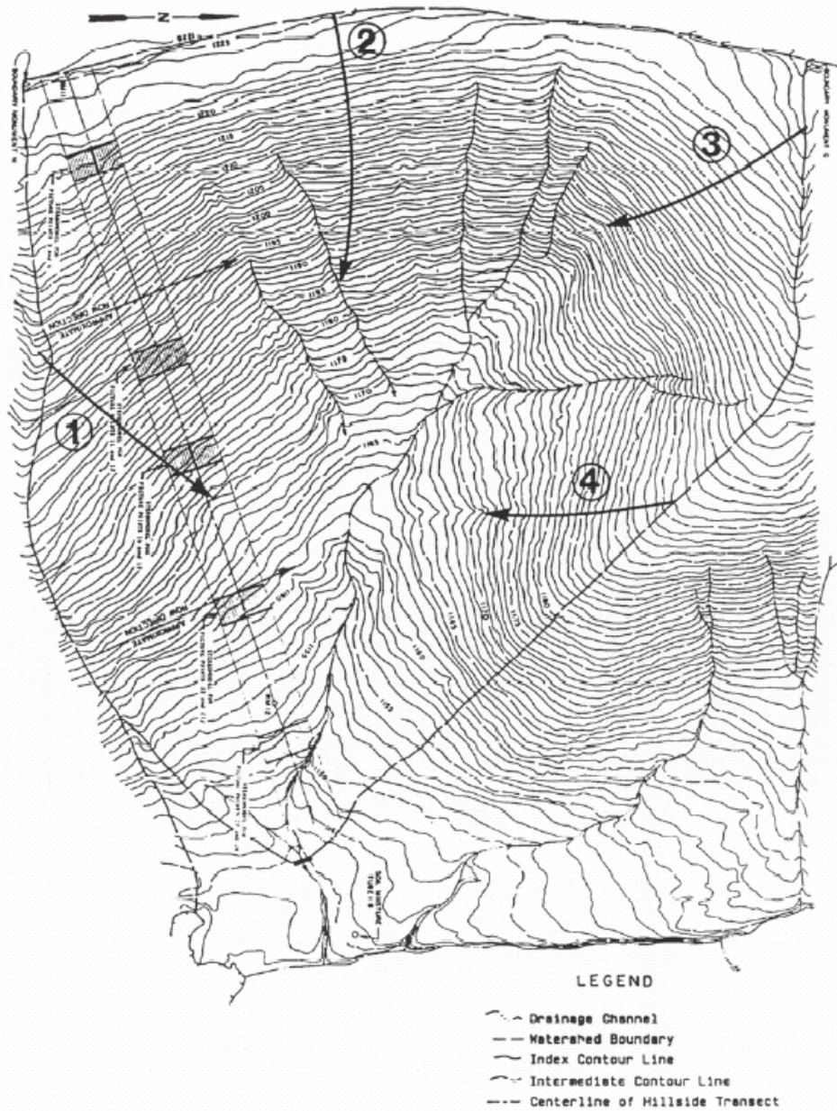
Slopes 2, 3 and 4 end at concentrated flow, while slope 1 ends at the point of deposition.
